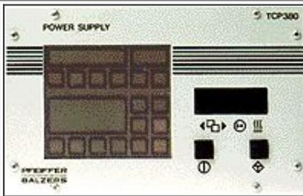
The image shows the control panel of a Pfeiffer Vacuum TCP380. It features a digital display, several buttons, and a power supply section. The text 'POWER SUPPLY' and 'TCP380' are visible at the top. The Pfeiffer logo and 'VACUUM' are at the bottom left. | <b>Für Pumpe:</b><br>alle TPH/TMH/U bis 520                                                                             |
